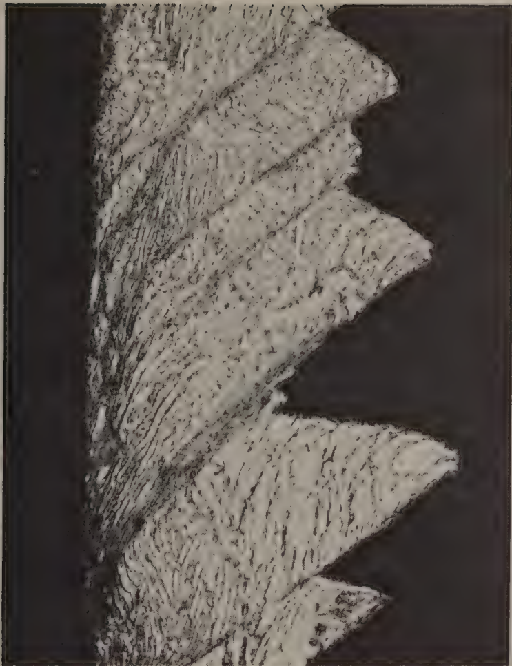
Fig. 8. Inhomogeneous titanium chip. a.) Magnification, 400x
